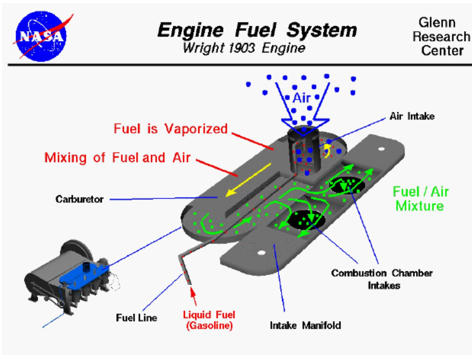
The fuel line continues past the valve, along the top of the engine, and into the the side of the **air intake** as shown on this figure. The liquid fuel drips into the **carburetor**, which is a flat, enclosed pan that sits on the top of the engine. The floor of the carburetor is hot because it sits over the engine cylinders. Air is drawn into the carburetor, through the air intake, because of the action of the pistons far downstream. During the [intake stroke](#) of the engine,
