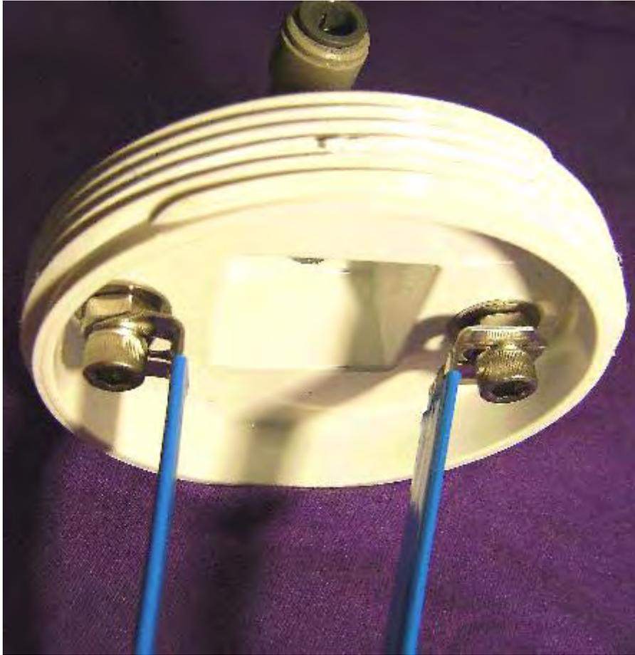
In order to ensure that the stainless steel straps are tightly connected to the electric wiring, the cap bolts are both located on the robust, horizontal surface of the cap, and clamped securely both inside and out. A rubber washer or rubber gasket is used to enhance the seal on the outside of the cap. If available, a steel washer with integral rubber facing can be used.
