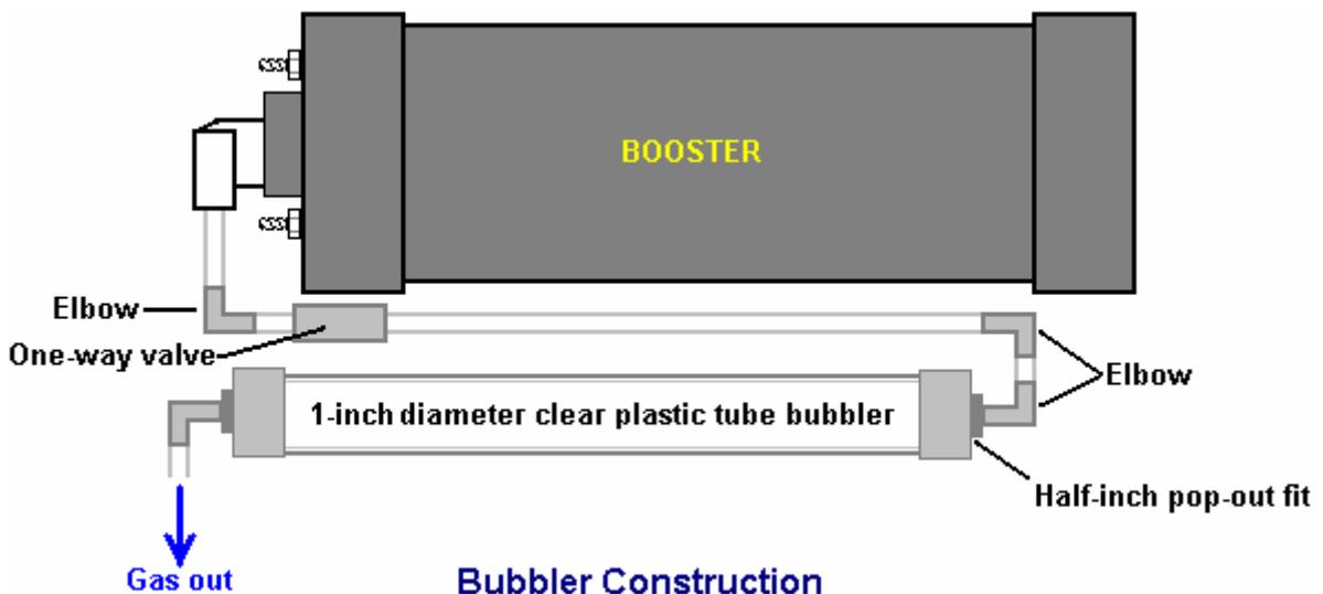
The half-inch diameter elbows at the ends of the one-inch diameter bubbler tube have their threads coated with silicone before being pushed into place. This allows both of them to act as pressure-relief pop-out fittings in the unlikely event of the gas being ignited. This is an added safety feature of the design.
