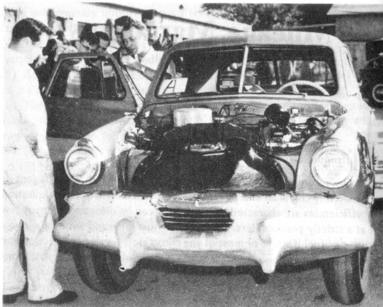
Plate 12.1 A modified 1947 Studebaker which achieved 149.95 mile/US gal in the 1949 Wood River competition
