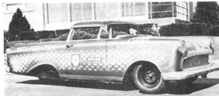
Plate 12.3 A modified 1959 Opel which achieved 376.59 mile/US gal in the 1973 Wood River competition
