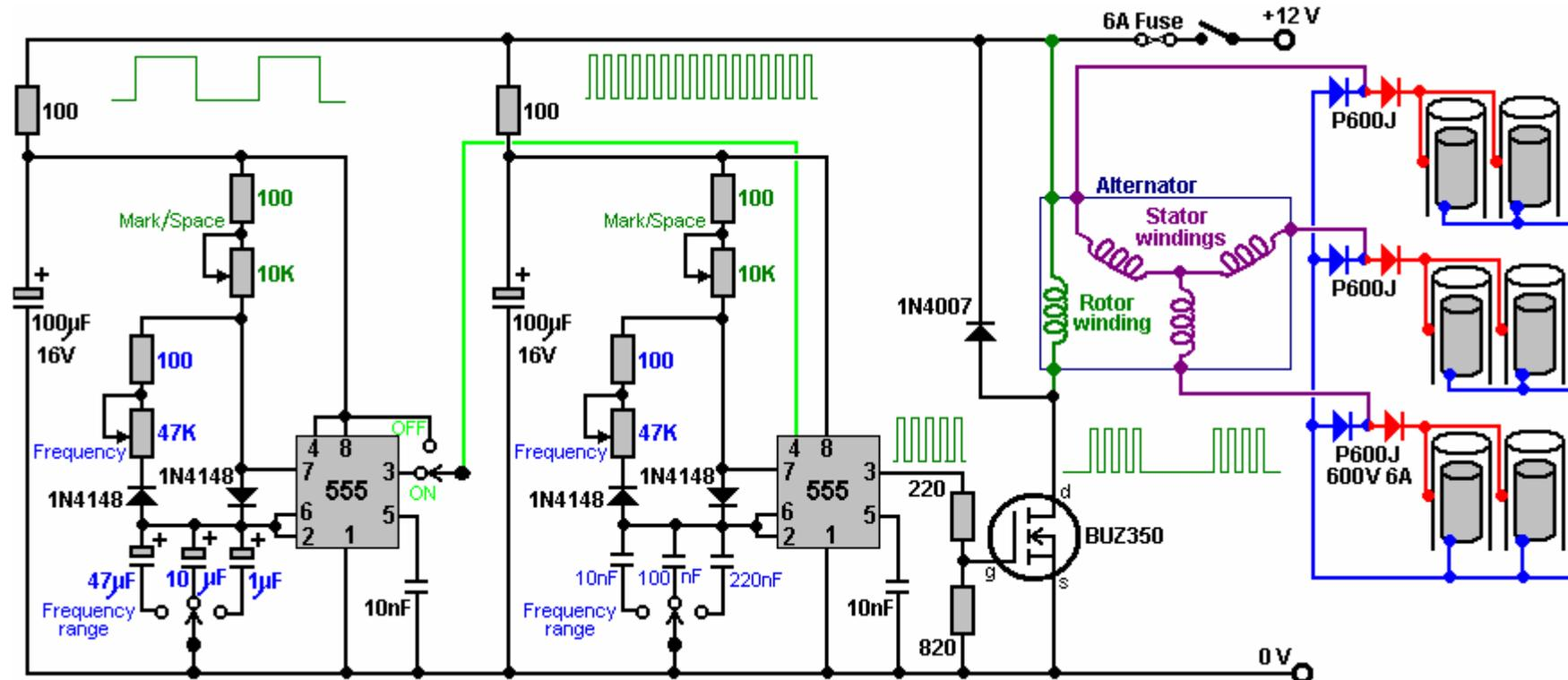
In this rather unusual circuit the rotor winding of an alternator is pulsed via an oscillator circuit which has variable frequency and variable Mark/Space ratio. The oscillator circuit has a degree of supply de-coupling by the 100 ohm resistor feeding the 100 microfarad capacitor. This is to reduce voltage ripple coming along the +12 volt supply line, caused by the current pulses through the rotor winding.
